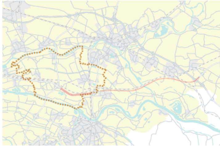
Figure 1. Construction plan A15 (author; Projectbureau ViA15, n.d.): Current connection between Valburg and Ressen will be widened to 2x3 lanes and the A15 will be connected to A12.
