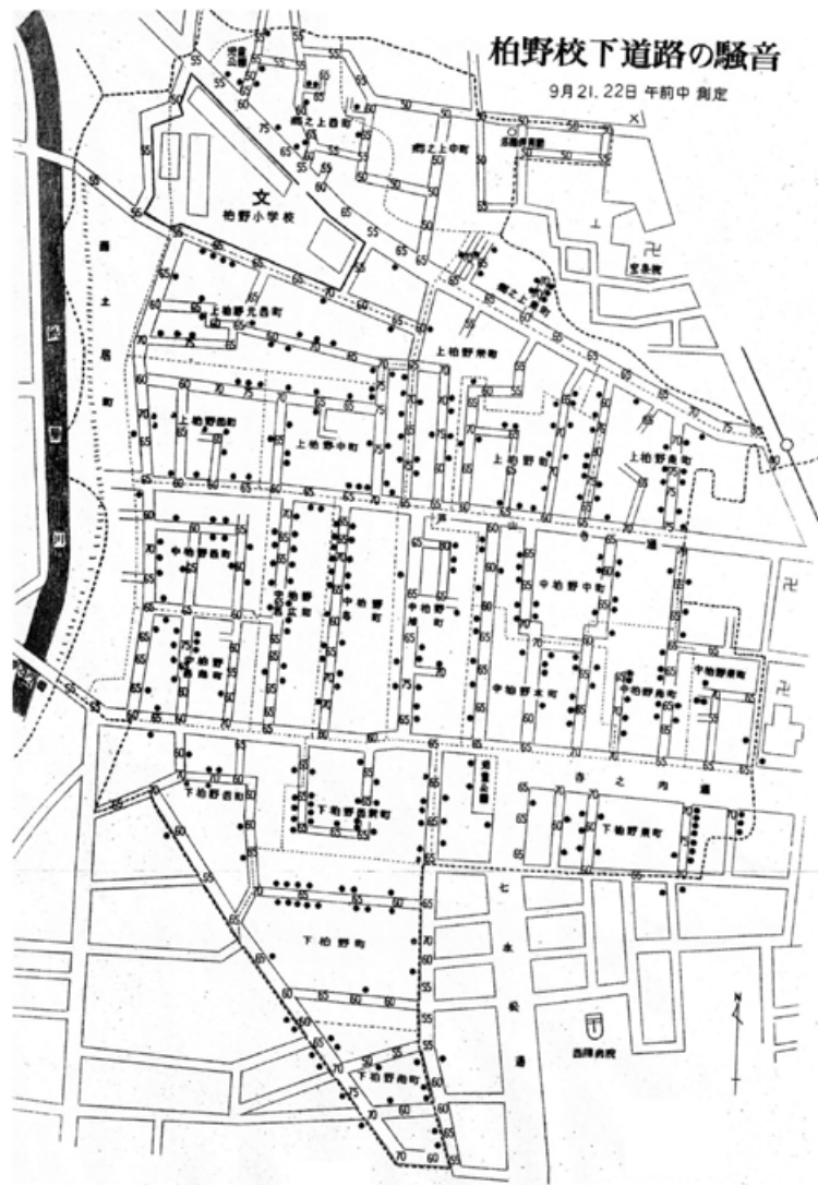
Figure 2. Measurements of sound levels and locations of the weaving noises (September 1965) in Nishijin no Ko to Hata no Oto (1966). The numerical values show sound levels (in dB), and the dots show the locations of the residential houses from which weaving noises were audible.
